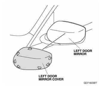
While applying light pressure against the left door mirror cover, carefully remove the seven adhesive backings as shown. Then, firmly press the left door mirror cover against the left door mirror.
